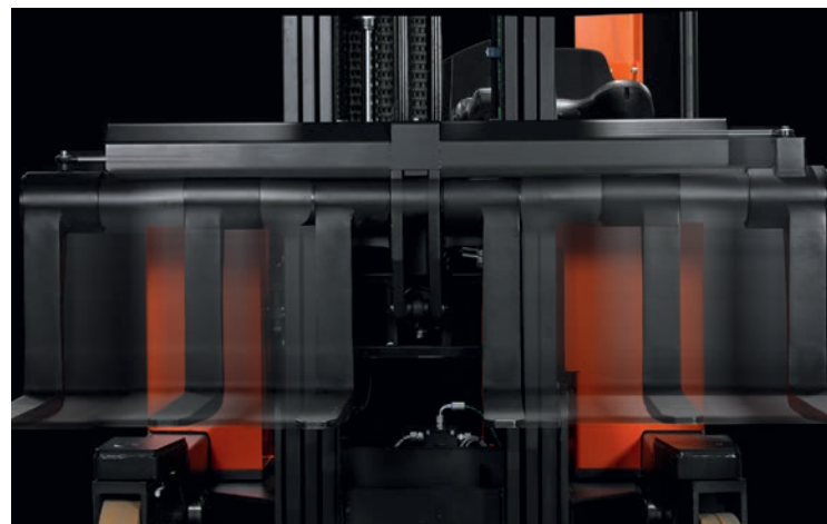
BT Reflex F-series' hydraulic fork spreader quickly adapts the truck to loads of different dimensions
