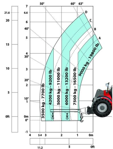
Machine on tyres with winch 9000 kg (Metric)
