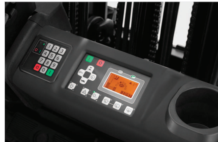
Multifunction display gives key information at a glance, as well as allowing the parameter settings to be adjusted to suit the needs of the application
