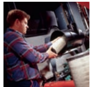
The air filter is easily accessible under the bonnet.
