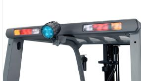
Toyota designed rear LED lights for improved driver visibility and safer handling operations.
