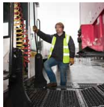
Wide stairways, sturdy handles and even rear deck increase productivity and safety.
