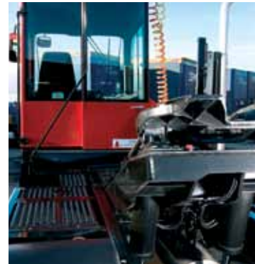
Two double-acting hydraulic cylinders for faster trailer lifting and lowering.
