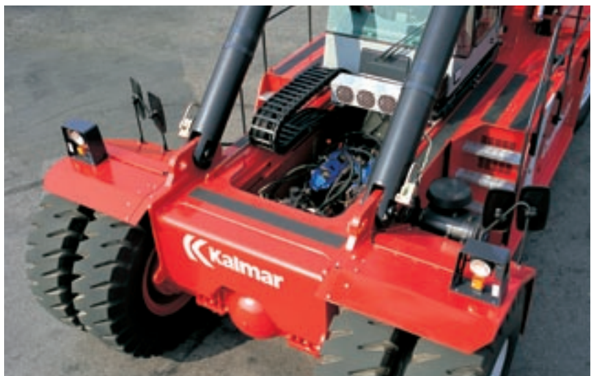
Easy access for inspections- and maintainance work when top covers are removed.
